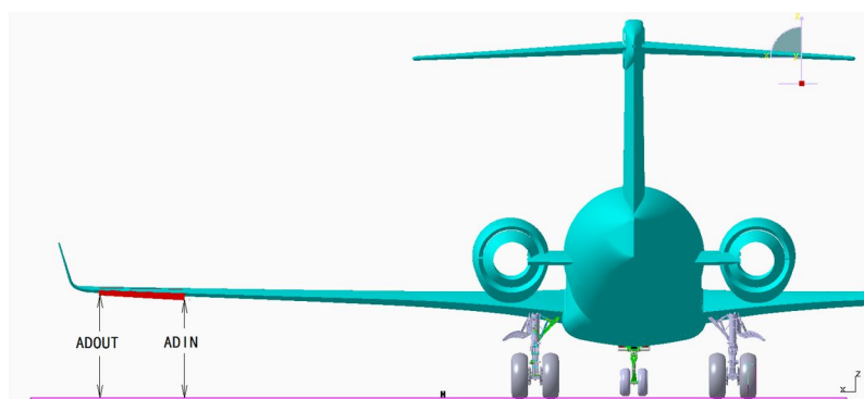
Figure 6 Ground Clearances at Aileron Down Status (Sheet 1 of 1)
